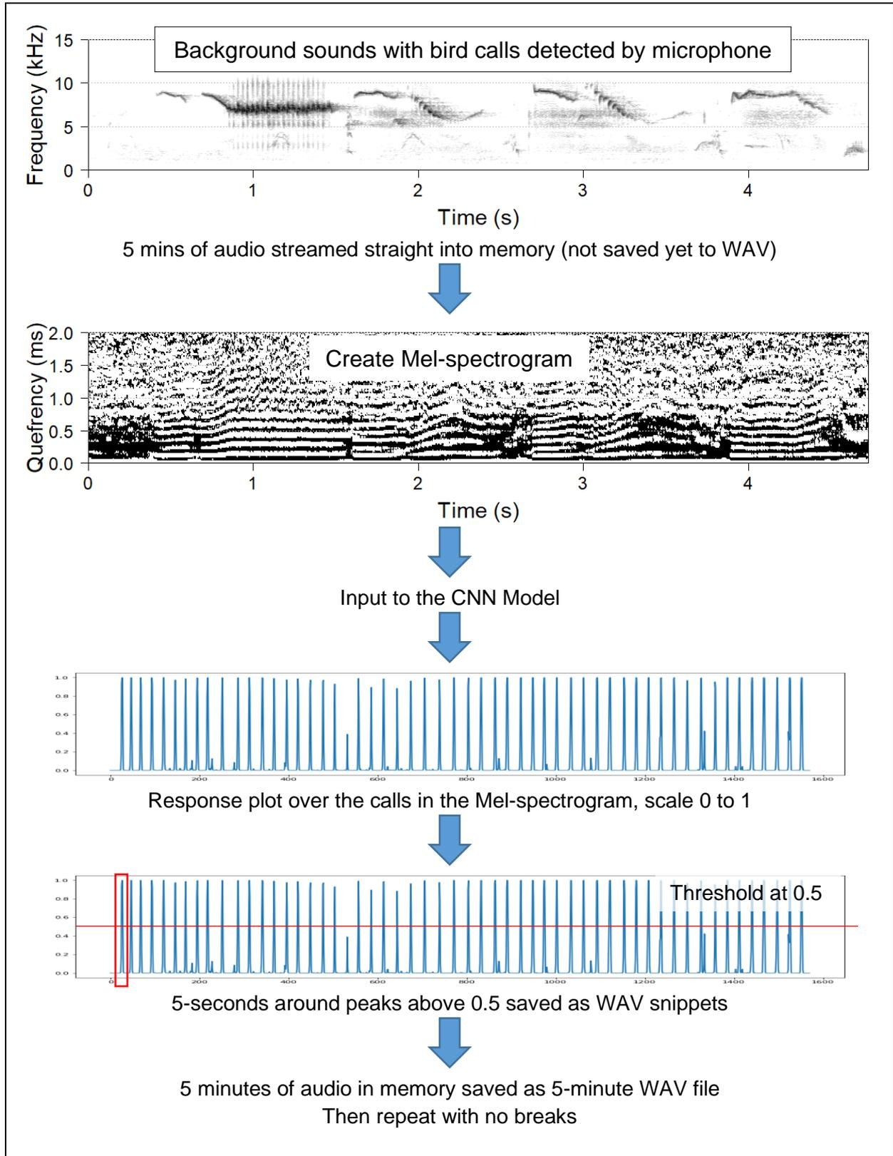
Figure 2. Illustration of what happens on the prototype recording device.
