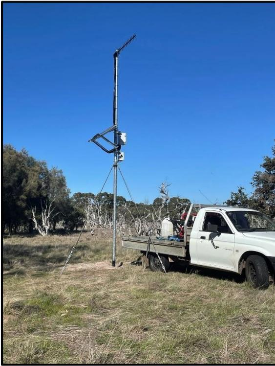
*Figure 8. a) Automated recording unit (ARU) with two omni-directional microphones positioned beneath Lithium-Ion solar charged battery. Split conduit piping surrounds exposed cabling to provide protection from wildlife. b) Four guy wires ratcheted to one tonne of pressure hold the 6m galvanised central mast (c) which supports the ARU, battery, solar panel and Yagi antennae.*
