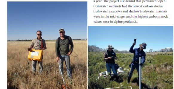
Left: The field team measuring greenhouse gas concentrations using the Los Gatos Research (LGR) Ultra-portable Greenhouse Gas Analyser (Deakin University Blue Carbon Lab)
